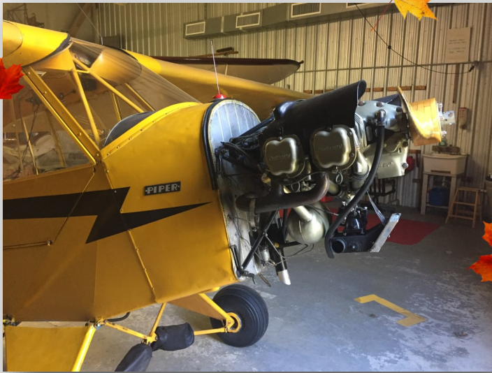
Dave Liebman found out a badly decomposed muffler is what led to smoke in the cockpit on his Cub's last flight thanks to Gino's professional investigation.
